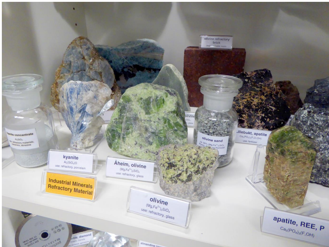
Figure 1. Exhibition display showing the industrial minerals olivine and kyanite, their processed concentrates (in glasses) and one application (olivine refractory brick used for smelter paneling). Source: NGU.
