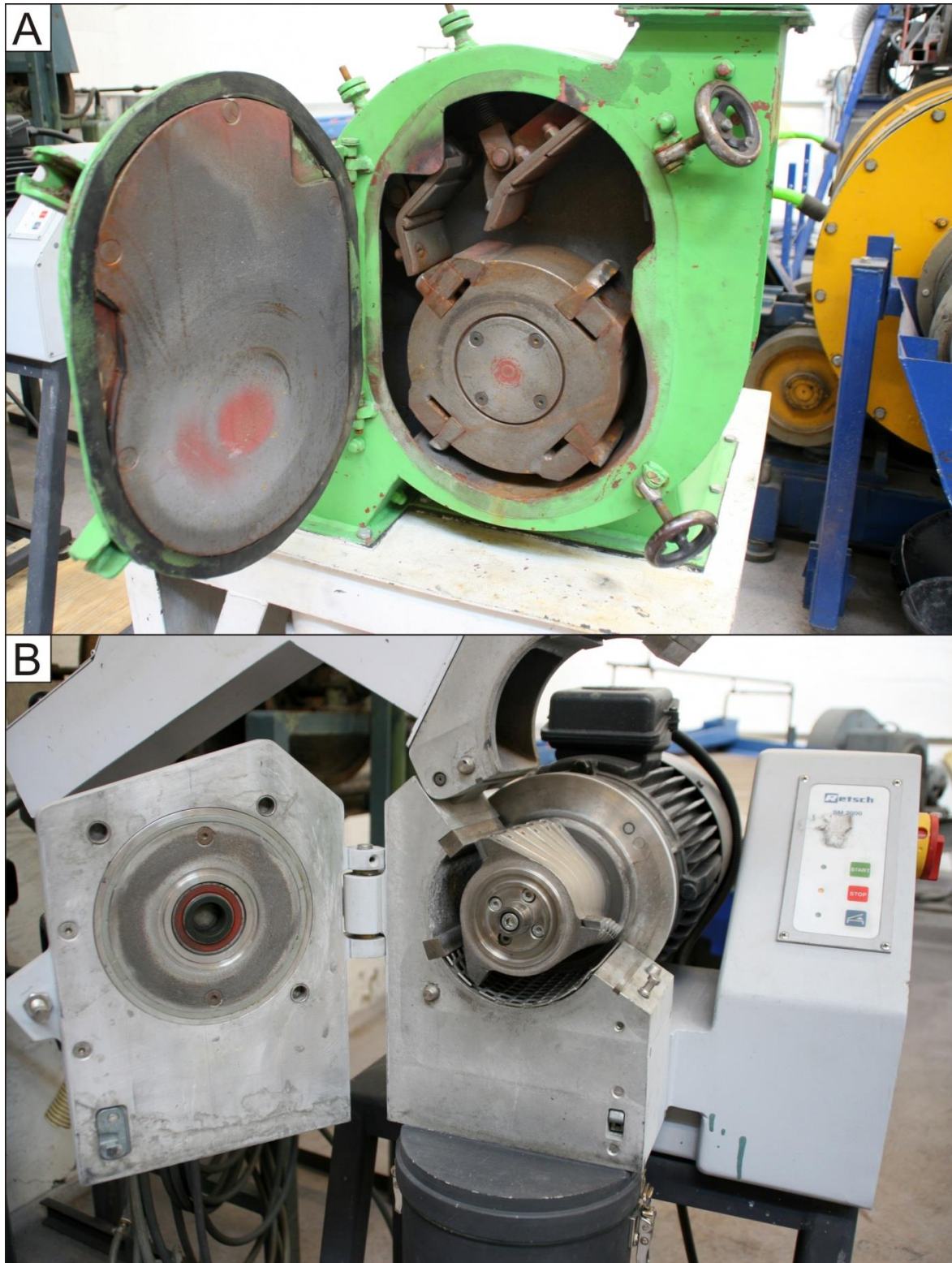
Figure 8. Crushers used for crushing compact cameras and mobile phones. A - Hazemag Impact Crusher for dry material 0-100 kg/h. B - Retsch SM 2000 Shredder. Source: NGU.
