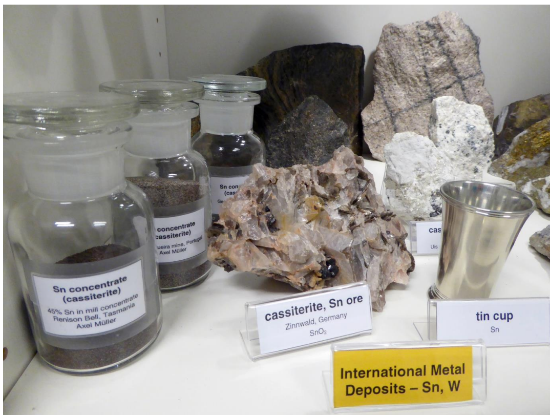
Figure 2. Exhibition display showing the base metal minerals cassiterite (SnO 2 ), three examples of Sn concentrates (glasses to the left) and one application (tin cup). Source: NGU.
