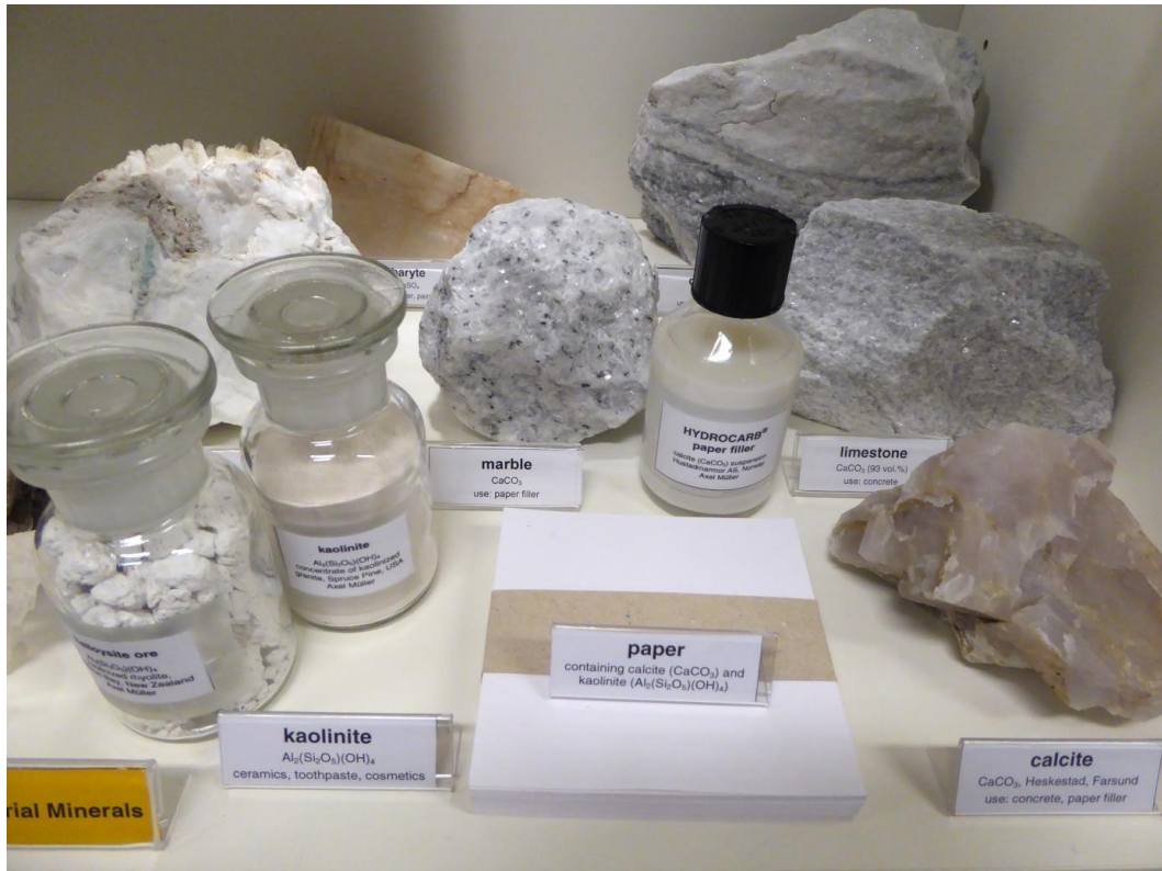
Figure 3. Exhibition display showing the industrial minerals calcite (limestone, marble) and kaolinite (glasses), one processing product (Hydrocarb paper filler) and one application (paper). Source: NGU.
