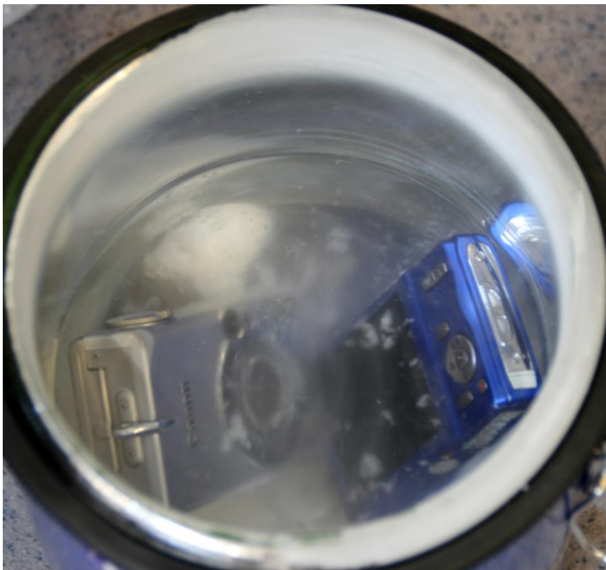
Figure 7. Compact cameras set in liquid nitrogen for 30 minutes prior to crushing. Source: NGU.
