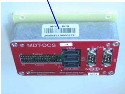
Figure 2. MDT-DCS module front panel connectors and labels.
