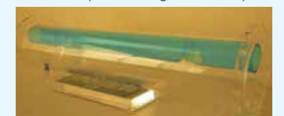
灰輸送設備【二重管】(写真は模型) Ash transport facility (double pipe) [The photo is of a model]
