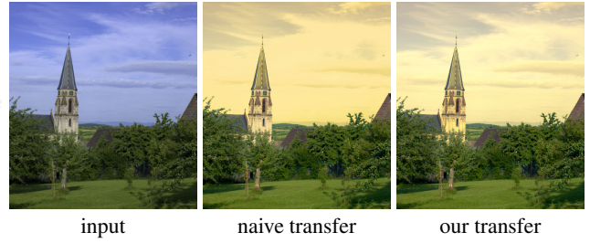
Figure 6: A naive transfer function that copies the color offset from the palette to every color in the image, even if clamped to remain in gamut, reduces dynamic range in the image (middle). Our transfer function (right) is able to make better use of the dynamic range. Photo courtesy of the MIT-Adobe FiveK Dataset [2011].
