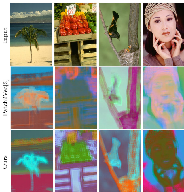
Fig. 6 Supervised vs. unsupervised embedding technique. Top: input images, from the training data of Ref. [3]. Middle: results of Patch2Vec [3]. Bottom: results of our unsupervised technique. Note that although our method did not train on these images, the textures are significantly less apparent in our embeddings. This suggests that segments with similar texture are embedded to closer locations in the embedding space.
