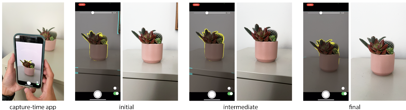
Figure 1: We present a photography guidance tool implemented as a capture-time app. Our tool allows the user to analyze the current clutter in the scene, and adjust until they achieve an image with less clutter. Here we show a sequence of overlays that the user sees as they make intermediate adjustments from their initial framing to achieve their final image. For the initial and final images, we show the overlay on the left and the corresponding photo on the right. The user notices the corner of the painting peeking into the photo in the initial frame, shifts the camera to the left to remove it from frame, but still notices the additional clutter caused by the strong line on the shelf in the foreground of the image in the intermediate frame. The user repositions the plant to the corner of the shelf to achieve the final image with a clean background.
