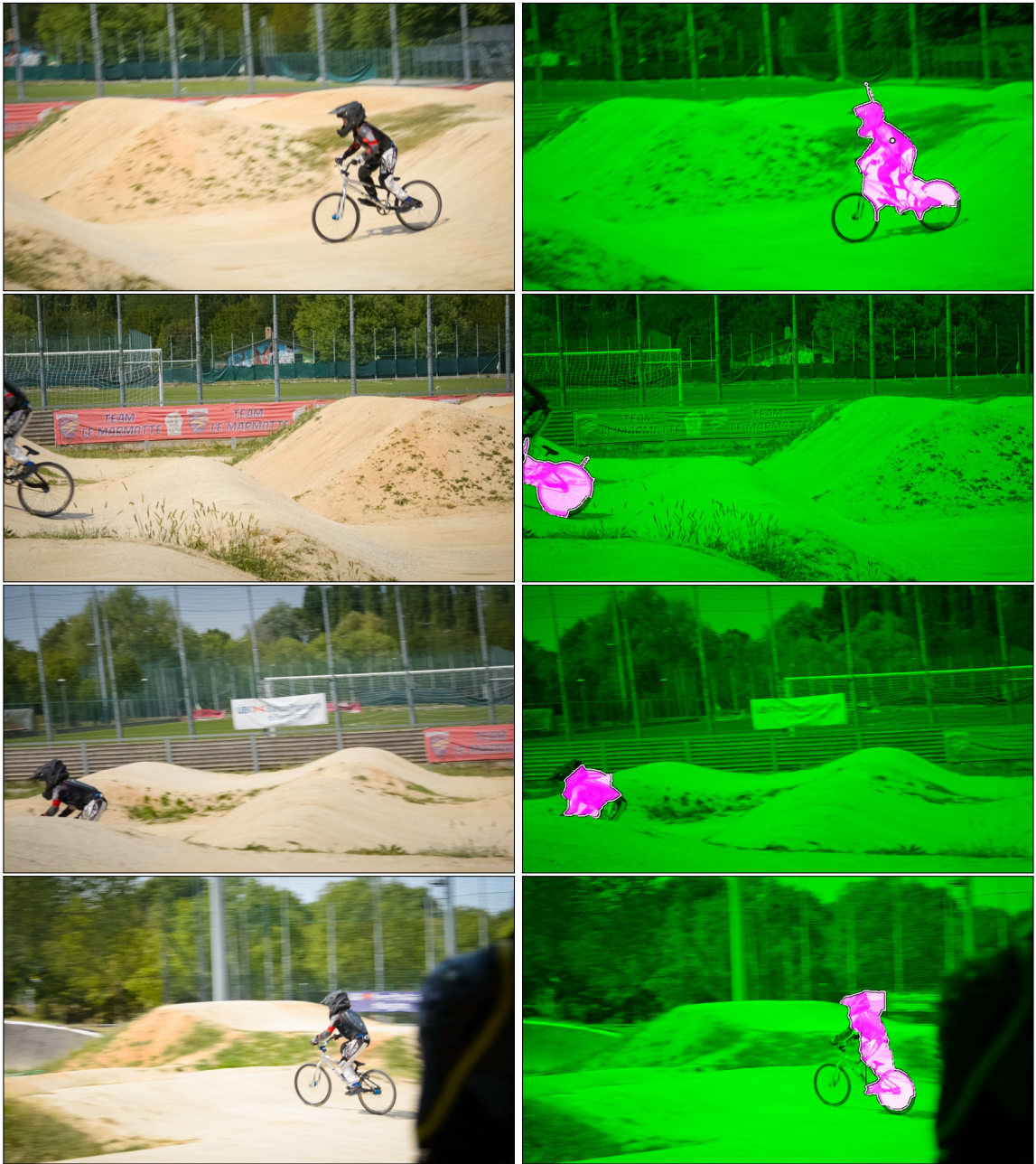
Figure 2.7: Single-click multi-frame selection. Given an input video (showing frames 0, 33, 50, 81), the user clicks on a single seed point (white dot, top-right image). We segment all images using distances to this single seed point. Notice how we can select the object without explicit template matching, despite appearance changes and occlusions. This demonstrates the universality property of our embedding.
