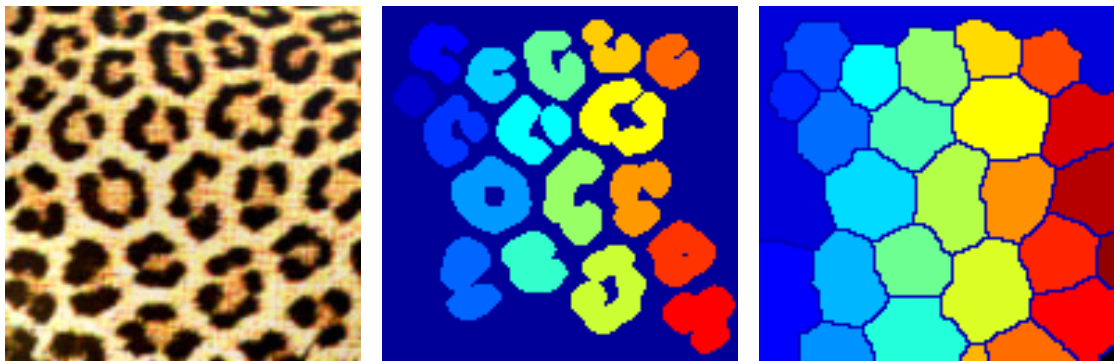
FIGURE 4.4: Left: original image. Middle: particles extracted using color difference thresholding. Right: maximal usable area for particle blending. Each cell contains a single particle together with as large a border as possible, to facilitate blending into the background.
