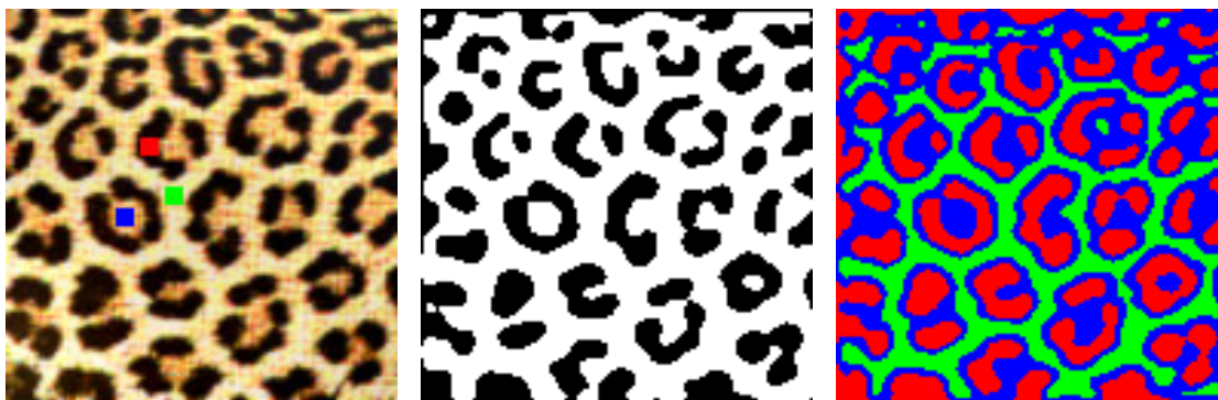
FIGURE 4.1: One possible way to extract background pixels. The user specifies an area which is background and an area which is particles (two clicks total, shown as green and red squares on the left image) and the thresholding mechanism produces the result shown in the middle. More degrees of separation can be created. A separation into 3 categories is shown on the right image (user required to click on 3 locations: green, red and blue squares on left image).
