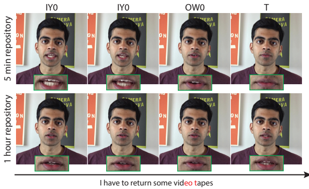
Fig. 10. Effect of small repository size. As shown here, the result from the 5-minute repository look less temporally stable as the transition from IY0 to OWO is more drastic than the result from the full-hour repository. With 5-minute repository, the actor also has an incorrect closed-mouth at T because we do not have as good a selection of phoneme coarticulations with a small repository as we do with a full-hour one.
