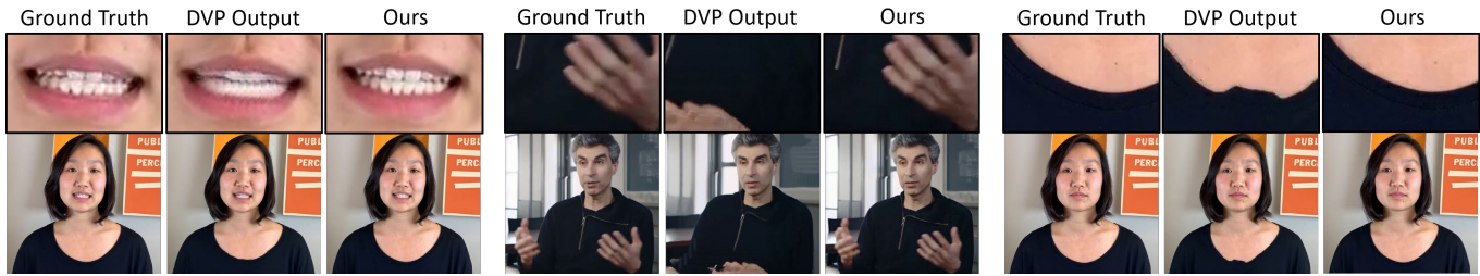
Fig. 8. Comparison of different neural face rendering backends: We compare the output of our approach with a baseline that is trained based on input data as proposed in Deep Video Portraits (DVP) [Kim et al. 2018b]. DVP does not condition on the background and thus cannot handle dynamic background. In addition, this alternative approach fails if parts of the foreground move independently of the head, e.g., the hands. Our approach explicitly conditions on the background and can thus handle these challenging cases with ease. In addition, our approach only has to spend capacity in the mouth region (we also re-weight the reconstruction loss based on a mouth mask), thus our approach gives much sharper higher quality results. Video credit (middle): The Mind of The Universe.
