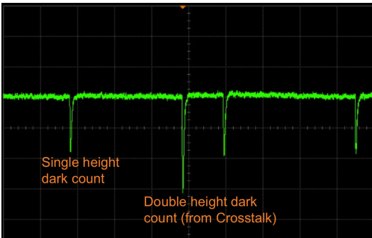
Figure 21. Oscilloscope Shot Showing Dark Counts
