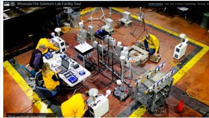
Missoula Fire Lab's Combustion Chamber floor and sampling hood that will be used for this study's emissions testing in the laboratory.
