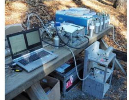
Missoula Fire Lab and Sonoma Ecology Center will do field tests using a similar emissions test process (shown above: field testing at CALFIRE Alta Forestry & Fire Protection Station, CA). 1
