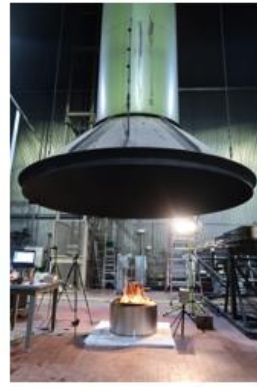
Missoula Fire Lab's Combustion Chamber floor and sampling hood that will be used for this study's emissions testing in the laboratory.
