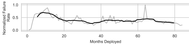
Fig. 2. Moving average (black) of raw (gray) normalized failure rates vs. DDR4 DIMMs’ deployment time in production. Failure rates tend to stay constant over a 7-year period.
