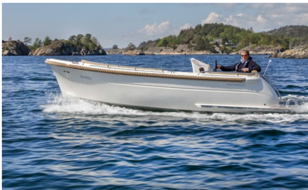
GreenWaves 601 is an all-electric Norwegian motorboat. The standard motor is 7.5 kW and the standard lithium battery pack allows 5-7 peaceful hours at sea. Photo: Johner Bildbyrå AB
