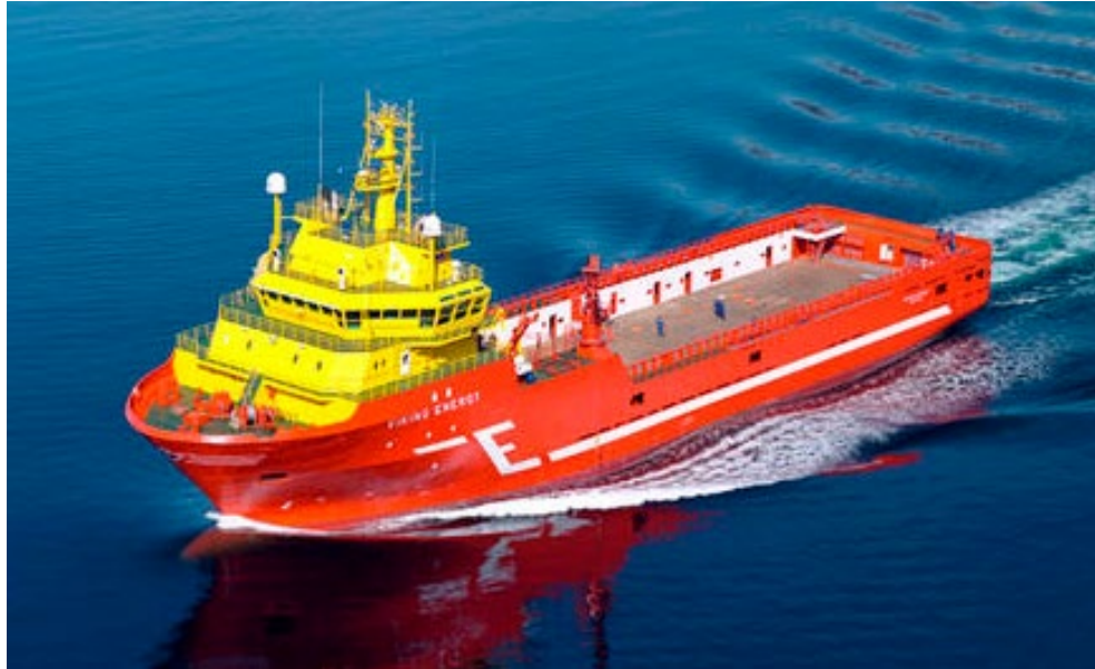
Eidesvik's supply vessel Viking Energy was launched in 2003 as the first LNG-powered offshore vessel. The ship made history again in 2016, when it was fitted with an advanced battery system that has reduced annual fuel consumption by 17 %. The battery system has a capacity of 650 kWh/1600 KW. Photo: Eidesvik Offshore
