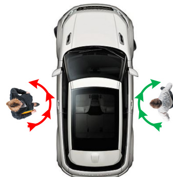
Fig. 2: Driver (right) and passenger (left); arrows show direction of turning during entry (driver: clockwise and passenger anticlockwise).
