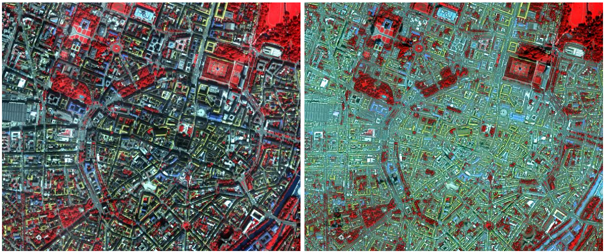
Figure 1.7: De-shadowing of an Ikonos image of Munich.
