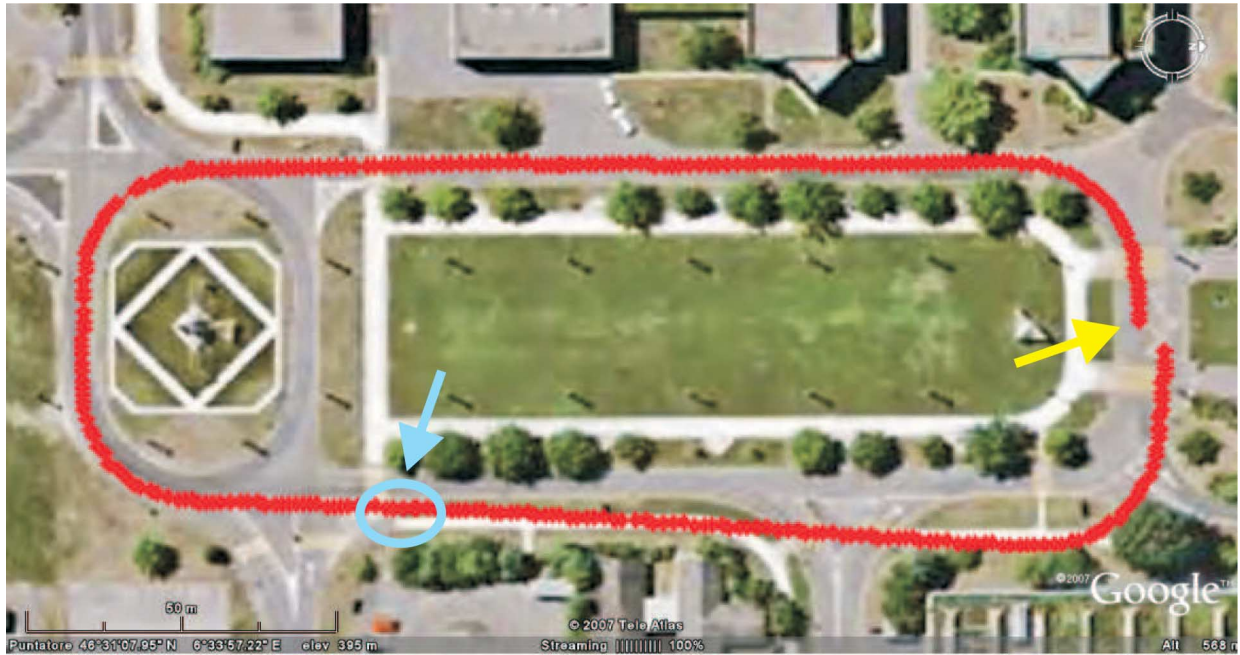
Fig. 16. Estimated path superimposed onto a Google Earth image of the test environment. The scale is shown at the lower left corner.
