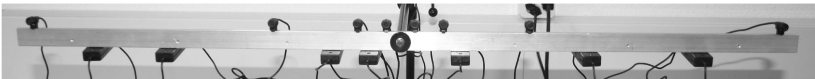
Figure 2.5: Eight channel microphone array used for audio acquisition in the ETHDigits dataset.
