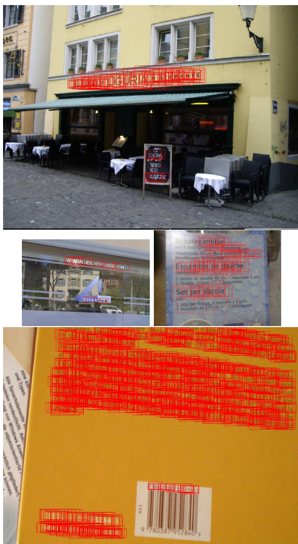
Figure 5.24: Raw detection results: All results correspond to the highest ROC curve in Figure 5.23. Note the handwritten text in the topmost line, rotated text, and gradient in the 2nd and 3rd image, respectively, and the large amount of text handled in the last example. The number at the bottom is not detected due to the lack of spacing to the barcode.
