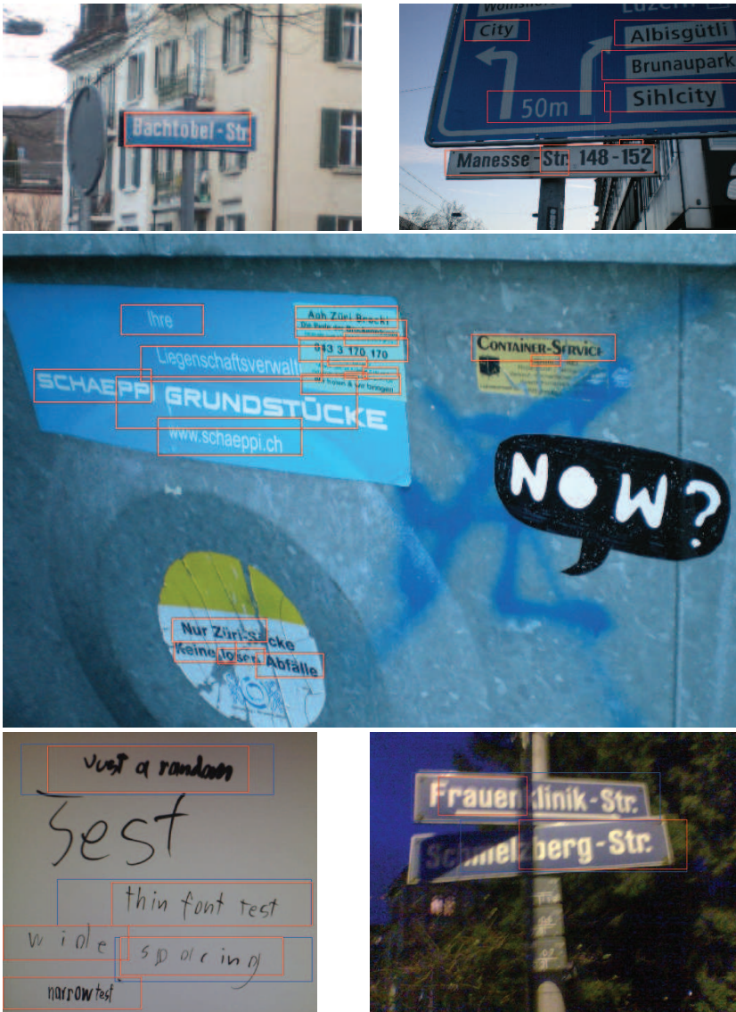
Figure 5.28: Example detections (I). True positives in red, false positives in blue. Note the variety of viewpoints and fonts, including handwritten text.
