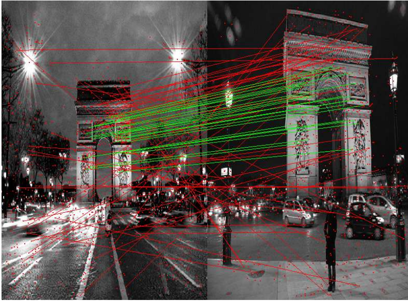
Figure 4.5: Feature matching with Homography. SURF feature matches are shown in red, inlying matches for the estimated homography in green.
