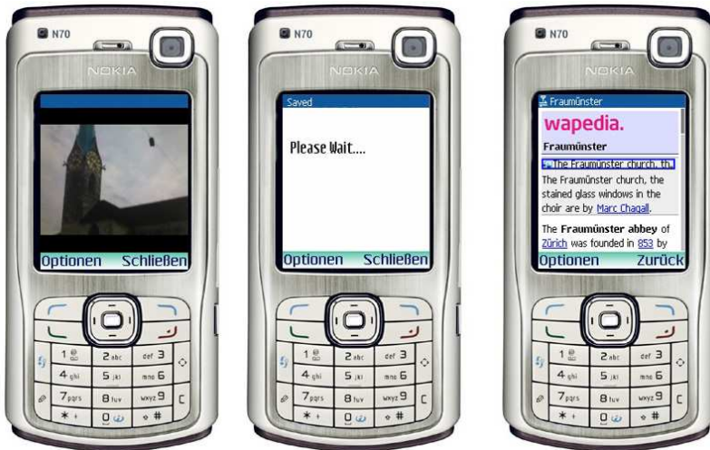
Figure 5.11: Client software for the cityguide application: the user snaps a picture, waits a few seconds, and is redirected to the corresponding Wikipedia page.
