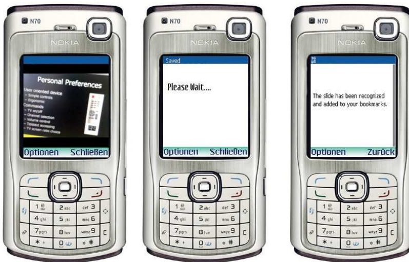
Figure 5.7: The user "tags" a presented slide using our mobile application by taking a picture (left), which is automatically transmitted to the server and recognized (middle), a response is given in an automatically opened WAP browser (right).
