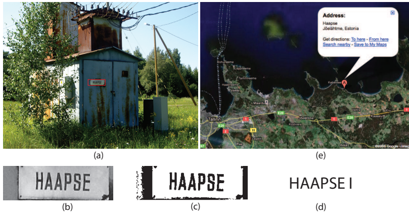
Figure 5.34: Guessing location from text in images. (a) Where was this picture taken? Detected text is labeled with the bounding box. (b) Close-up of the text. (c) After binarization. (d) Text returned from OCR. (e) Result when sending the text from (d) to Google maps. The picture was taken by the author of this thesis in the small village Haapse, Estonia, indeed.
