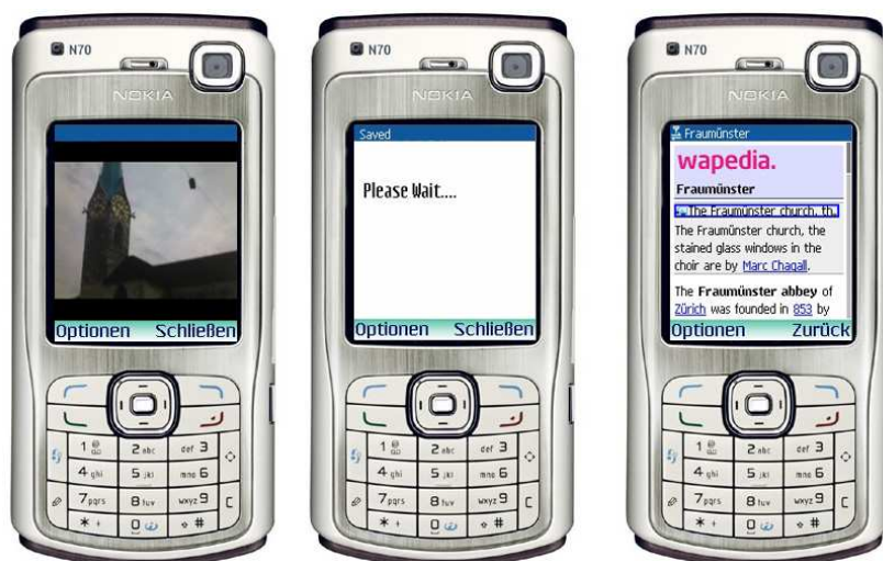
Figure 5.3: Client software for the cityguide application: the user snaps a picture, waits a few seconds, and is redirected to the corresponding Wikipedia page.
