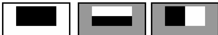
Figure 5.18: The intensity based features used. The absolute intensity difference between the black and the white region is calculated. Left: comparing block to window intensity; right: Haar-like edge features
