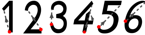
Figure 6.3: Single stroke gestures c = 1, \dots, 6 . The dot marks the start and finish-point of the trajectory described by the hand movement when drawing the number in the air. The dashed lines mark the section of the trajectory necessary to achieve an identical start and finish-point. The arrow indicates the direction of the movement.
