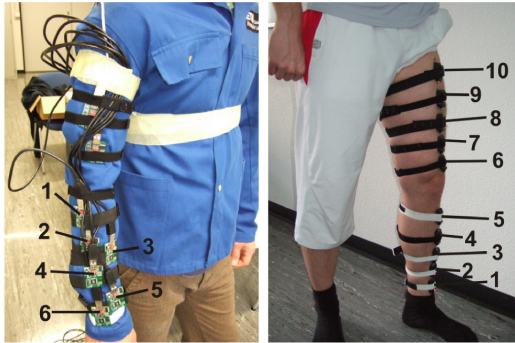
Figure 3.4: HCI scenario, left image: Six sensors are attached to the subject's right forearm. Fitness scenario, right image: Ten sensors are attached to the subject's left leg - five on the thigh and five on the lower leg.
