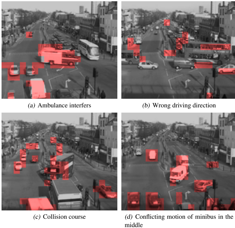
Figure 6.3: Detected anomalies that occurred in the scene. Conflicting Image regions are shaded in red.
