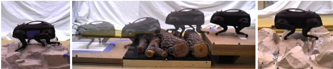
Figure 25: Boston Dynamics Inc. LittleDog quadruped robot, shown crossing several types of rough terrain. Images reproduced from [84].
