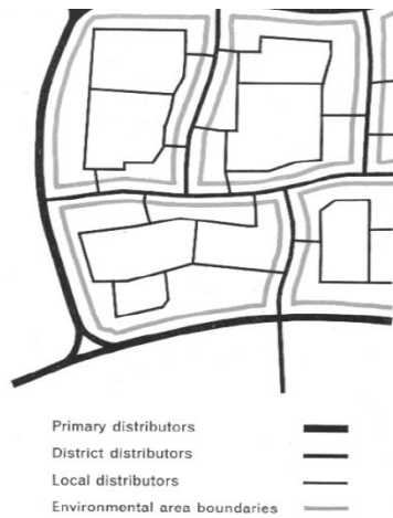
Figure 6: The Division between System of Traffic Distributors and a System of Environmental Areas Suggested in the Buchanan Report
