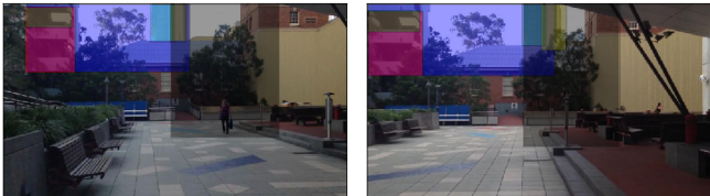
Fig. 4: Two example scenes from the Gardens Point Campus dataset with extracted and matched ConvNet landmarks. Notice the lateral camera displacement of several meters.
