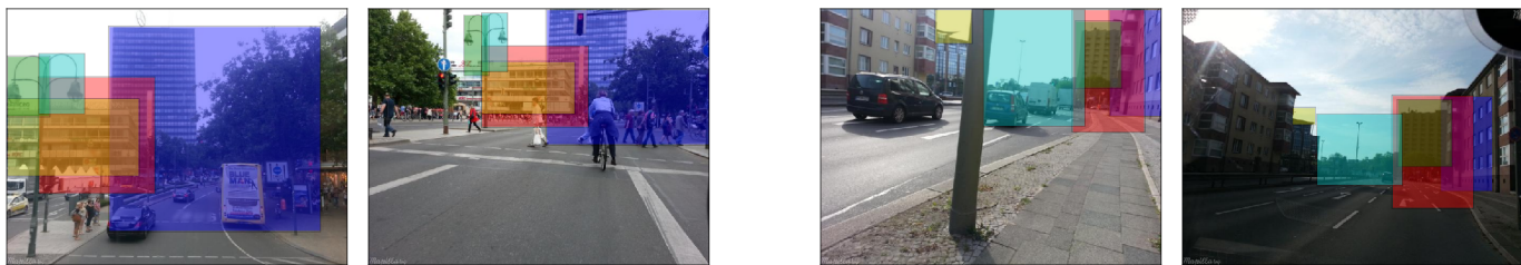
Fig. 1: We present a novel place recognition system that adapts state-of-the-art object proposal techniques to identify potential landmarks within an image. The proposed system utilizes convolutional network features as robust landmark descriptors to recognize places despite severe viewpoint and condition changes, without requiring any environment-specific training. The colored boxes in the images above show ConvNet landmarks that have been correctly matched between two significantly different viewpoints of a scene, thus enabling place recognition under these challenging conditions.
