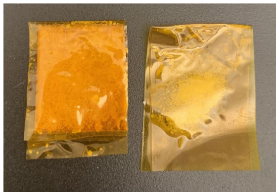
Figure 4.D.2. Example of good and poor sample-on-tape preparation practices. left: uniform sample on tape. right: non uniform sample
