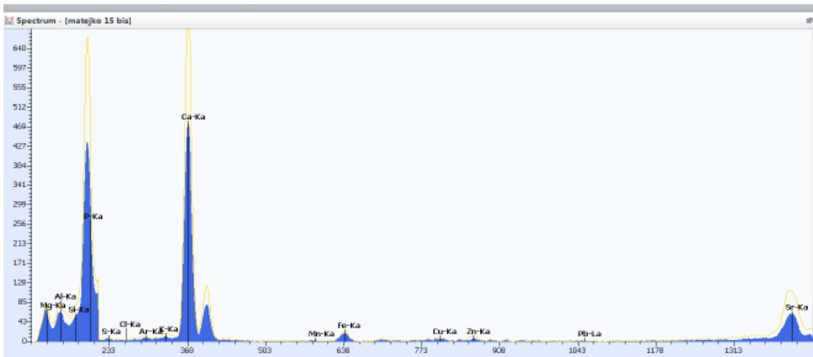
Fig. S38b. XRF spectrum of the Laque de Robert No. 6 paint sample compared with the Laque de Robert No. 5 spectrum (yellow line). Lesser amount of Ca, P and Sr were detected.
