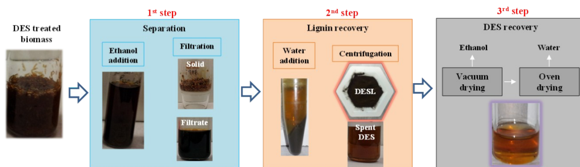
Figure S2. Procedure for pretreated solid, extracted lignin and DES recovery.
