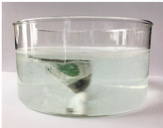
Figure S8. Washing durability of PVDF stitch textile sensor; Demonstration of the washing environment with commercial detergent by magnetic stirring.
