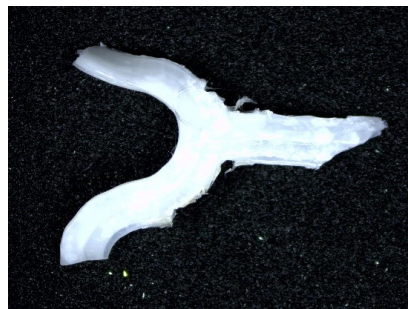
Fig.S9 Representative “Y”-shaped units of stent wreckage after degraded for 8 weeks.
