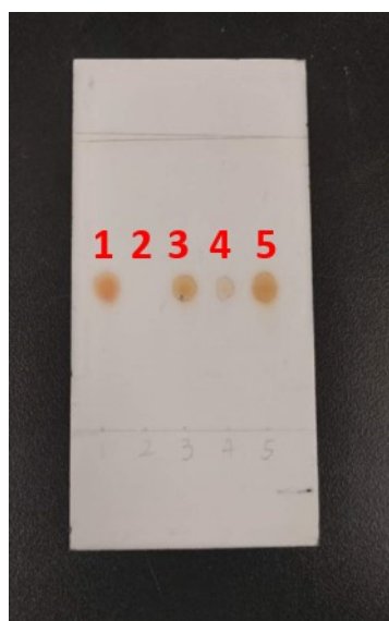
Figure S1. The TLC analysis results of different samples. 1-2: the standard sample of Ala and LA; 3-5: the reaction solution catalyzed by Ru/Ni@C (reactants: 3-LA, 4-glycerol, 5-pyruvate acid).
