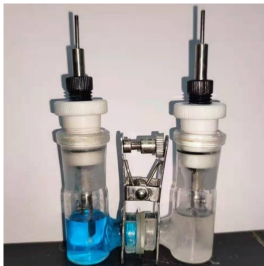
Fig. S42. Digital photo of the alkaline-acid hybrid Zn-Cu mould cell. The left tube contains the Cu metal electrode immersed in 1 M CuSO 4 (pH=1), the right tube holds the Sn-coated Zn metal electrode immersed in 6 M KOH + 0.3 M Zn(Ac) 2 , and the BM is used as the separator.
