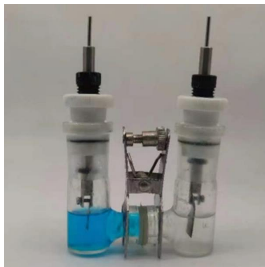
Fig. S26. The digital photo of the AEM Zn-Cu mould cell. The left tube contains the Cu metal electrode immersed in 1 M \text{CuSO}_4 ( \text{pH} = 1 ), the right tube holds the Sn-coated Zn metal electrode immersed in 2 M \text{ZnSO}_4 , and the AEM is used as the separator.
