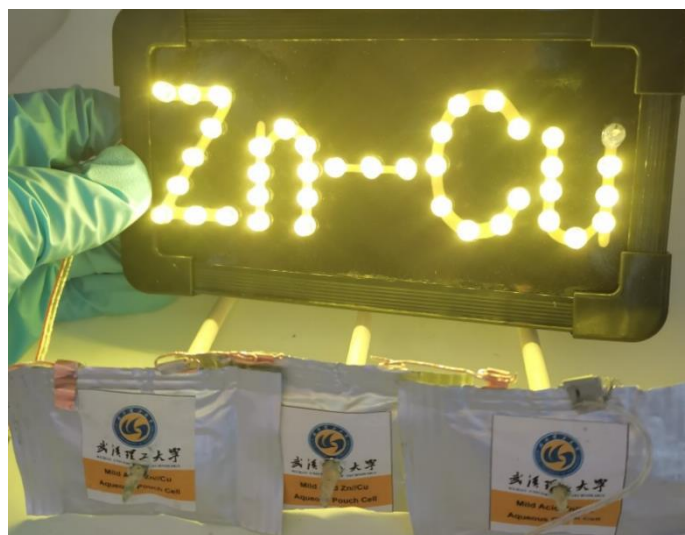
Fig. S40. LEDs lit by a series of three AEM Zn-Cu pouch cells after being punctured.
