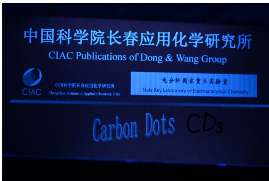
Figure S7. Digital photograph of the green diagram printed with the CDs ink under 365 nm UV irradiation after exposure to room light for 2 months.
