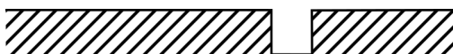
Figure 1.2: Black-box search style optimization landscape in which only a small region of the landscape is a lower energy than the remaining (flat) landscape.
