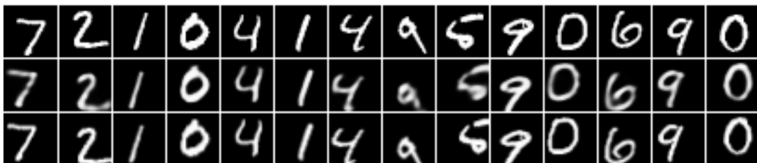
Figure 2.2: Reconstructions of translated digits using a transforming autoencoder with 100 capsules, each with 10 recognition units and 10 generative units. top row : input, middle row : reconstruction, bottom row : target output
