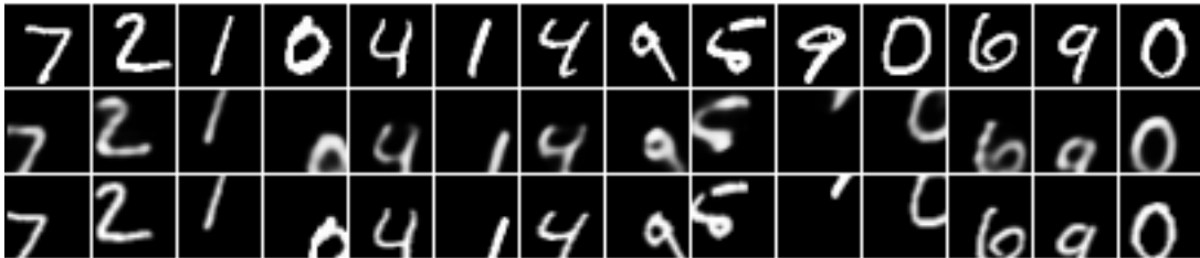
Figure 2.4: Reconstructions of translated digits using a transforming autoencoder with 100 capsules, each with 10 recognition units and 10 generative units. top row : input, middle row : reconstruction, bottom row : target output
