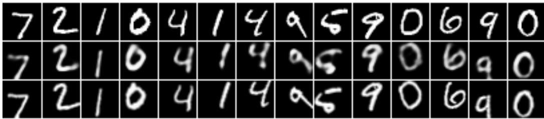
Figure 2.7: Reconstructions of translations and rotations of digits using a transforming autoencoder with 50 capsules, each having 20 recognition units and 20 generative units. Each capsule outputs x, y, \theta as instantiation parameters. top row : input, middle row : reconstruction, bottom row : target output
