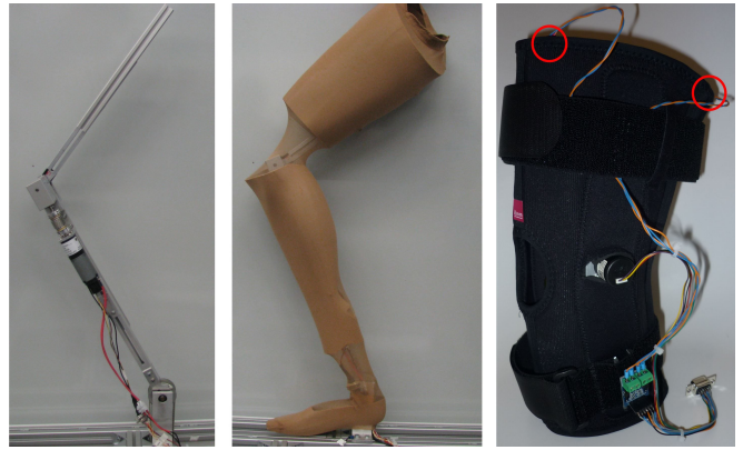
Fig. 3. Robot mechanics (left). Robot with cladding (middle). Interface orthosis (right, mirrored) with vibration motor positions (red circles).
