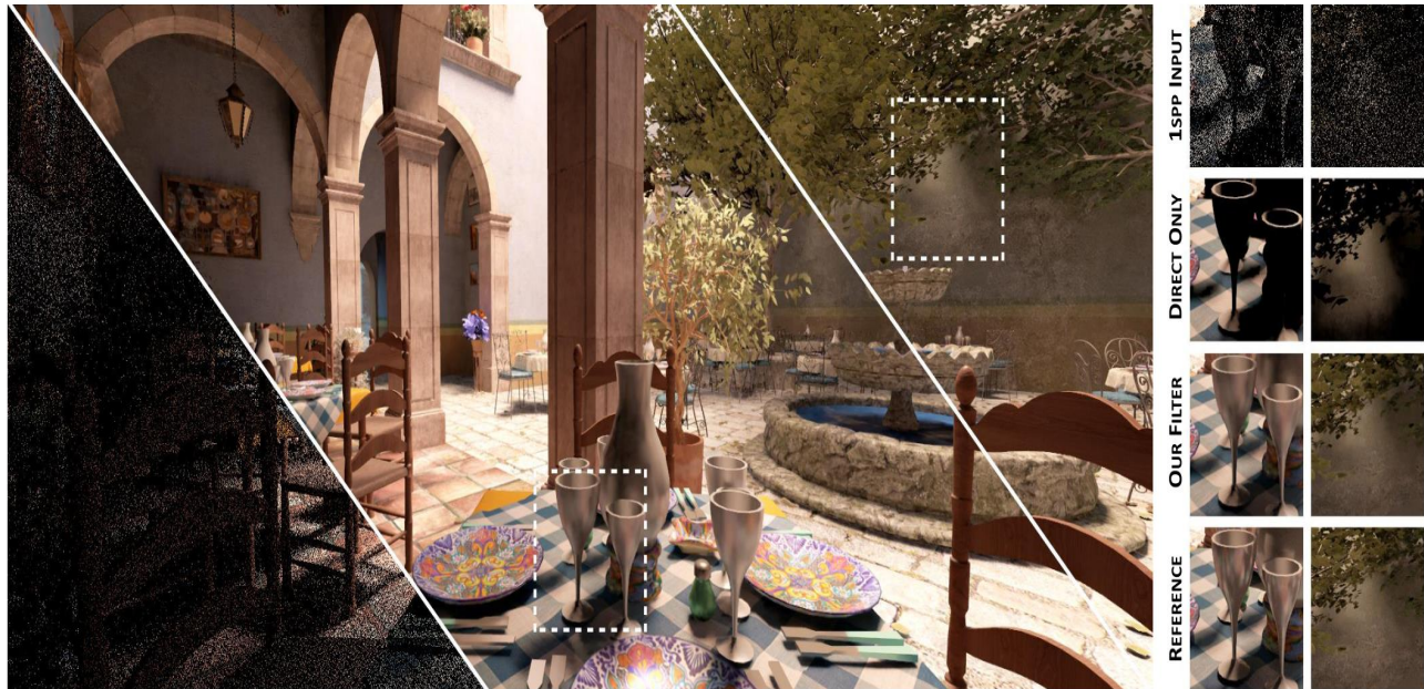
Figure 2: Representation of Monte Carlo Path Tracing with spatiotemporal variance-guided filtering to improve performance and rendering time from Schied et al. 6†
