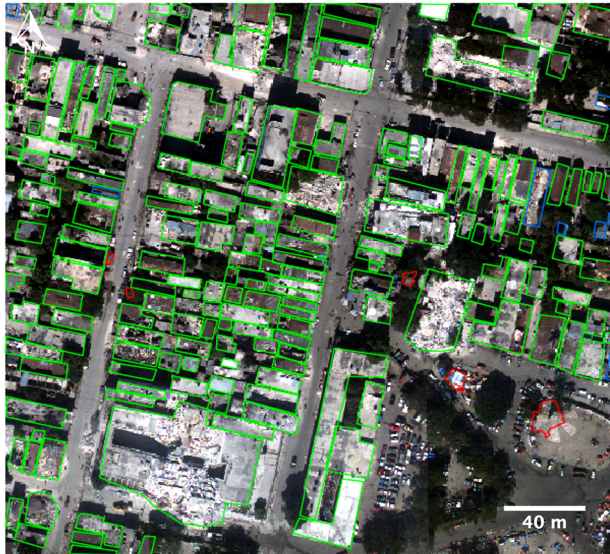
Fig. 9 Building segmentation results for a scene in Port-au-Prince. True positives are outlined in green, false positives are outlined in red, and false negatives are outlined in blue.
