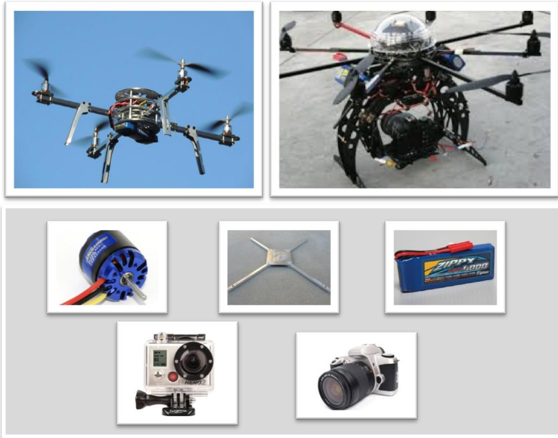
Figure 7: Typical quad copter UAV configurations. Top left: small machine; top right: big machine; bottom: typical structural elements and payloads.
