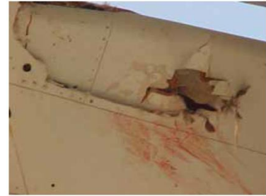
Figure 5: Damage to a Boeing 747 flap after a bird collision at 1200 feet AGL (Cleary, et al., 2006).
