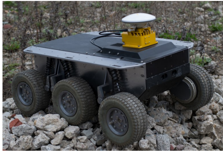
Figure 2: Duro Inertial sample installation
