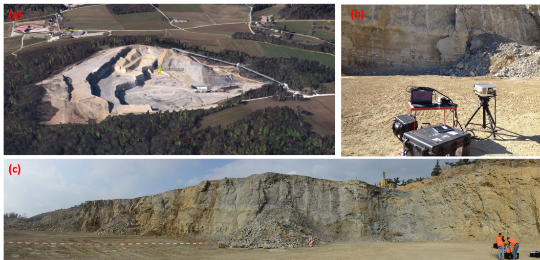
Figure 1. (a) Overview of the Jura Cement quarry; (b) the ground-based Telops Hyper-Cam instrument; and (c) photograph of the vertical cliffs.
