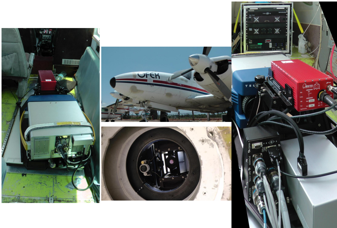
Figure 4 – Onboard installation of HyperCam sensor on the light aircraft. Left and right – Sensor installation inside the aircrafts; Middle-down – a view from below; Middle-up – a general view of the aircraft.
