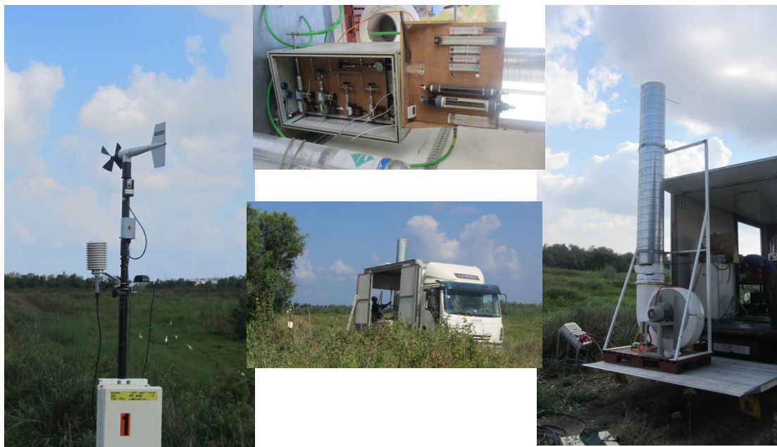
Figure 5 – Ground setup at release point. Left – on site meteorological station; Middle-down – release point; Middle-up – mass flow controllers; Right – release stack.
