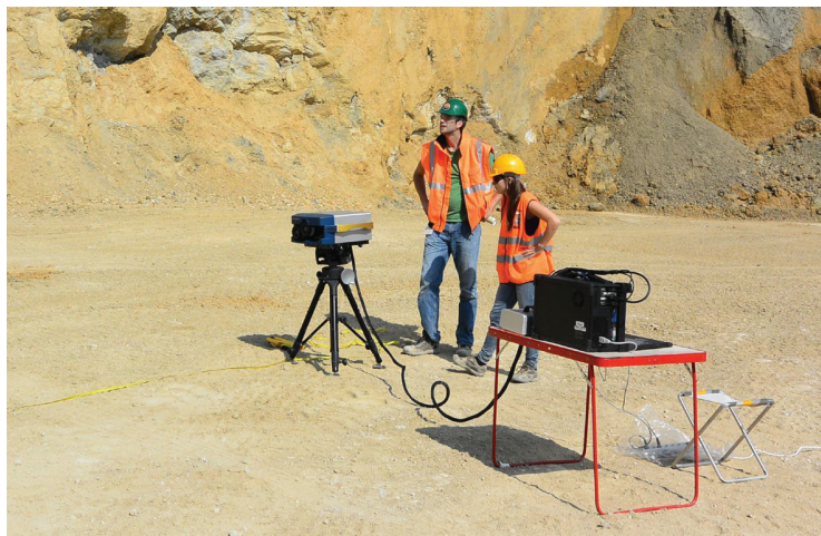
Figure 7. Proximal TIR sensor, Hyper-Cam, undertaking mine face mapping at the Jura cement quarry
