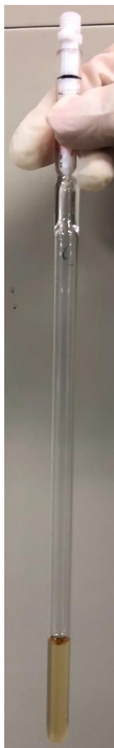
Figure S1. A reaction vessel for catalytic pentafluoroethylation of acyl fluorides (Wilmad-LabGlass 513-7PVM-9).
