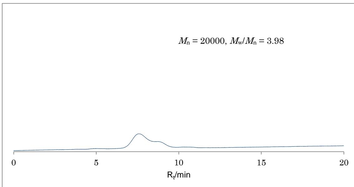
SEC profile of **3** (polymerization with LDA in the presence of MnCl<sub>2</sub> shown in Table 1)
