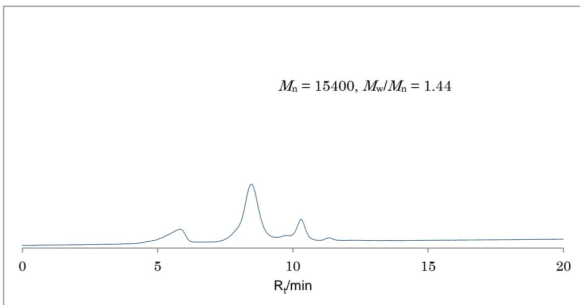
SEC profile of **3** (one-shot polymerization shown in Table )
