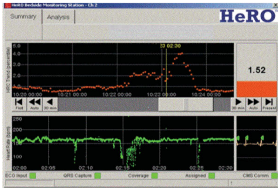
Fig. 1 Heart rate observation (HeRO) monitor-visualizing heart rate characteristics index, corresponding heart rate pattern, and controls to scroll forward and backward in time.
