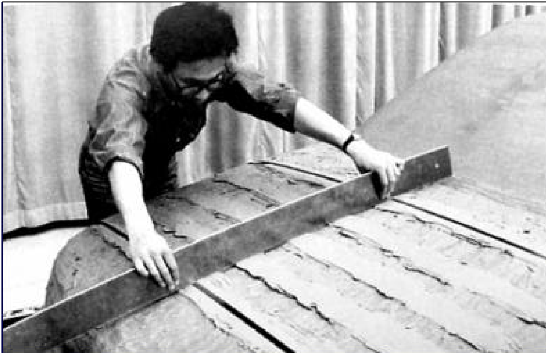
Figure 2.3: Physical curved tools. An artists sweeps out the surface of a clay model using a steel curve
