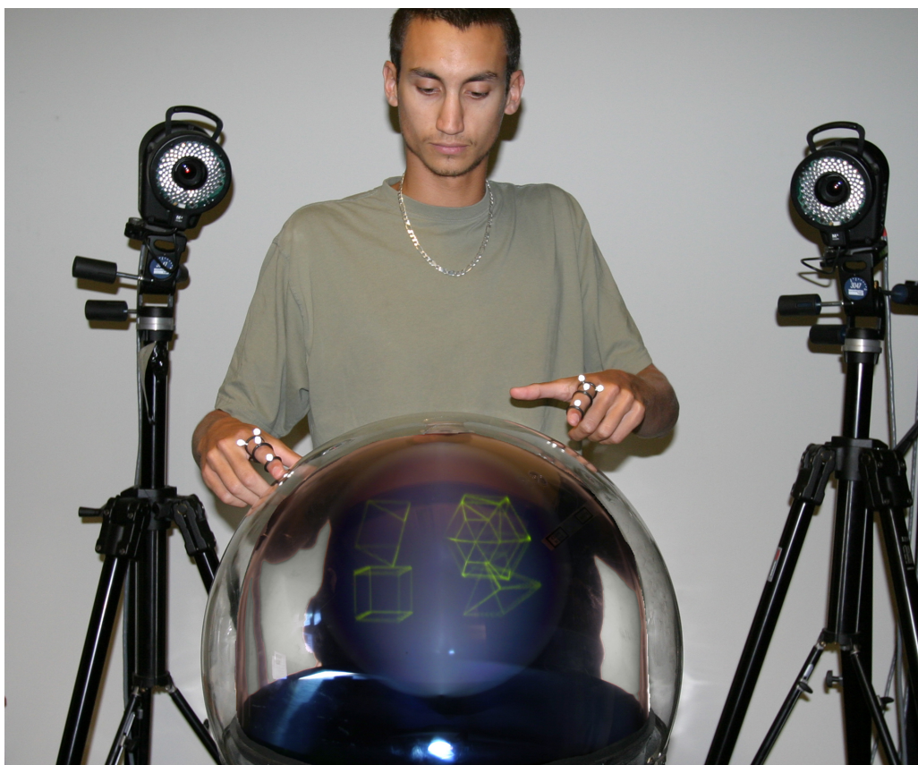
Figure 7-1. User working with a volumetric display, with finger input tracked using a camera-based motion tracking system.
