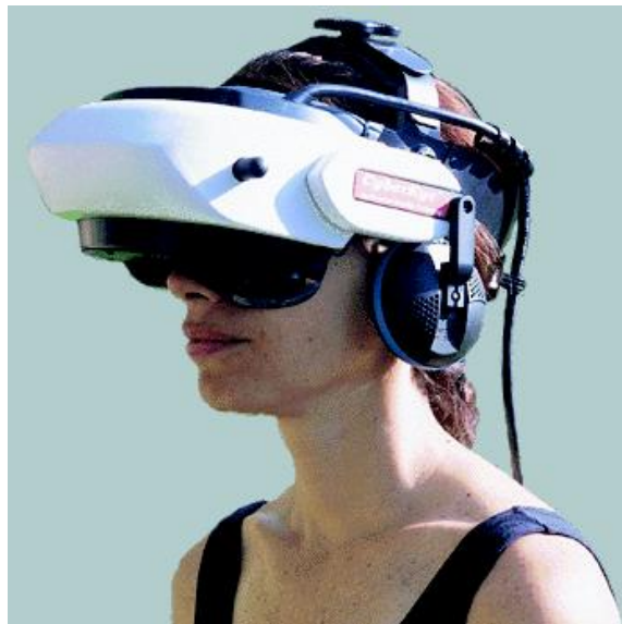
Figure 2-2. A head mounted display creates an immersive virtual reality by covering the user's eyes. Image taken from Buxton and Fitzmaurice [1998].
