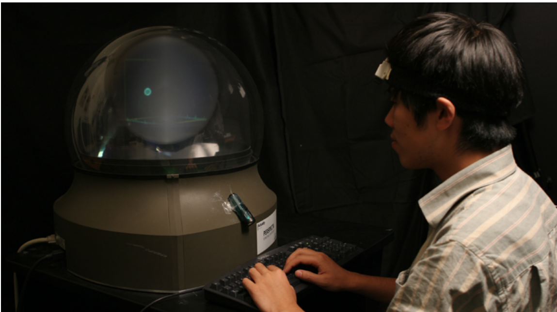
Figure 3-2. Volumetric display setup. The electromagnetic tracker measures head movement to allow imagery to be displayed only when head position is within a range.
