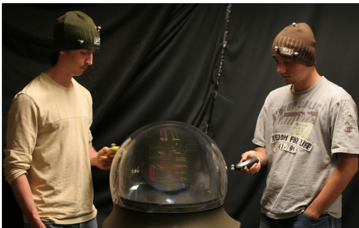
Figure 8-1. The prototype for our explorations allowed users to collaboratively interact with the volumetric display. Users' viewpoints and input devices were tracked in 3D.
