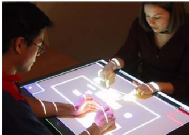
Figure 2-21. RoomPlanner application. Users collaborate using multiple hand and finger gestures on the table top display. Figure taken from Wu and Balakrishnan [2003].
