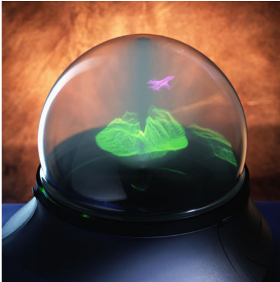
Figure 1-1. A 3D volumetric display. Voxels illuminated in true 3D space facilitate 3D viewing from anywhere around the display without wearing special glasses.
