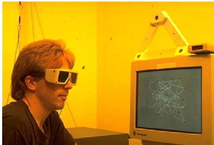
Figure 2-1. Fish tank displays combine stereoscopic and head tracking technology to create a viewing volume roughly equivalent to the inside of the monitor. Image taken from Ware and Franck [1996].
