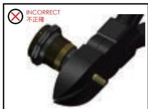
Please pre-thread the ball end hole by using a M3 Screw.
