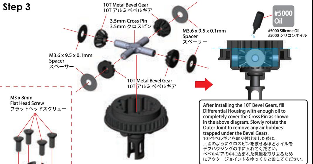
After installing the 10T Bevel Gears, fill Differential Housing with enough oil to completely cover the Cross Pin as shown in the above diagram. Slowly rotate the Outer Joint to remove any air bubbles trapped under the Bevel Gears.
