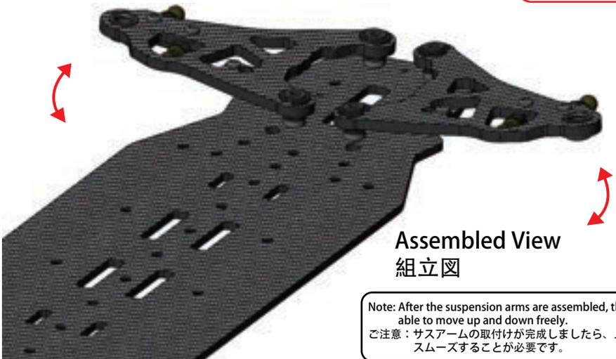
Note: After the suspension arms are assembled, they should be able to move up and down freely.
