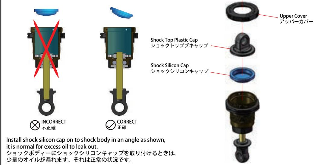
Install shock silicon cap on to shock body in an angle as shown, it is normal for excess oil to leak out.
