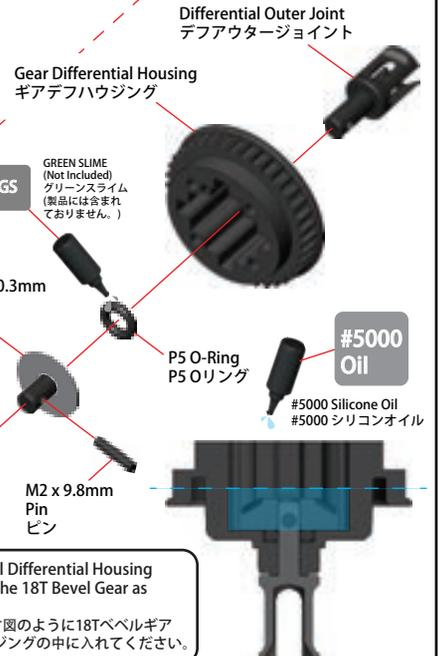
After installing the 18T Bevel Gear, fill Differential Housing with enough oil to completely cover the 18T Bevel Gear as shown in the right diagram.
