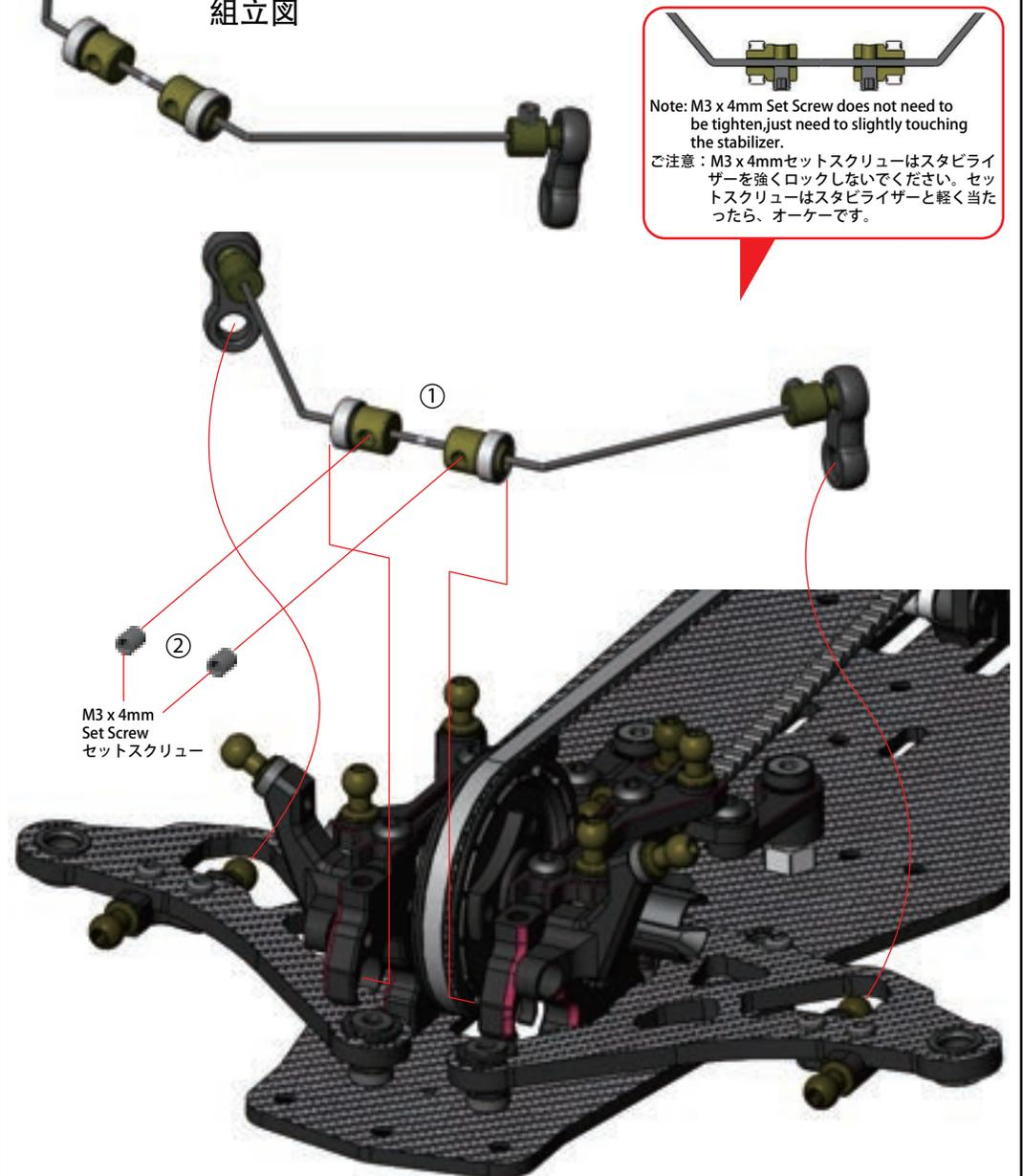
Note: M3 x 4mm Set Screw does not need to be tightened, just need to slightly touching the stabilizer.
