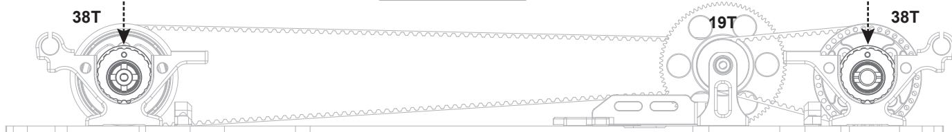
R11 2018 Internal Gear Ratio in 2.0 (19T/38T) (More Torque and acceleration)
