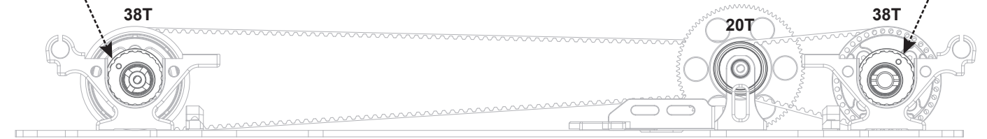
R11 2018 Internal Gear Ratio in 1.9 (20T/38T) (Smoother acceleration)
