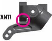
When adjusting steering on the radio, we recommend using full steering adjustment in order to get the best steering from the car. It is important to verify that the steering block does not touch the C-hub; that would lead to chassis tweak due to extra servo strain.
