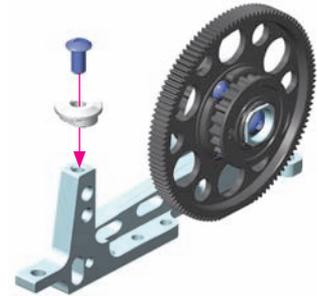
The top deck is connected to the motor mount via bushing. This setting provides maximum stability as it stiffens the entire car and eliminates flex to sides and front/rear.
