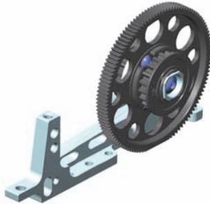
No bushing or bearing is used. This allows maximum flex and provides maximum steering. However, the car is less stable on-power.
